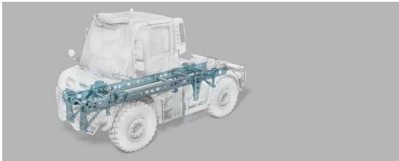
Four attachment and mounting areas: the Unimog implement carrier is one of the most productive work vehicles there is. Many different implements can be combined thanks to the standardised interfaces. These include the front mounting plate, attachment points on the frame, mounting brackets on the sides and at the rear as well as ball-point positions on the platform sub-frame.
