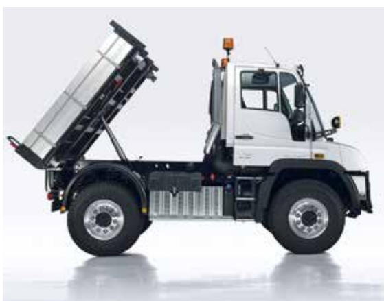
The separate tipping hydraulics allow tipper bodies or trailers to be tipped independently of the working hydraulics.
