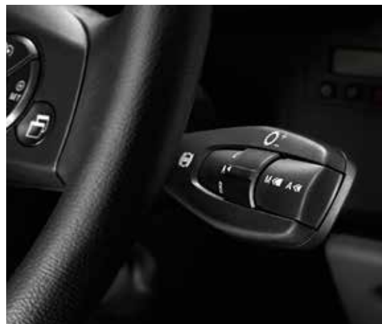
The steering column control on the right makes it easy to change gears. The premium engine brake is also operated from here.
