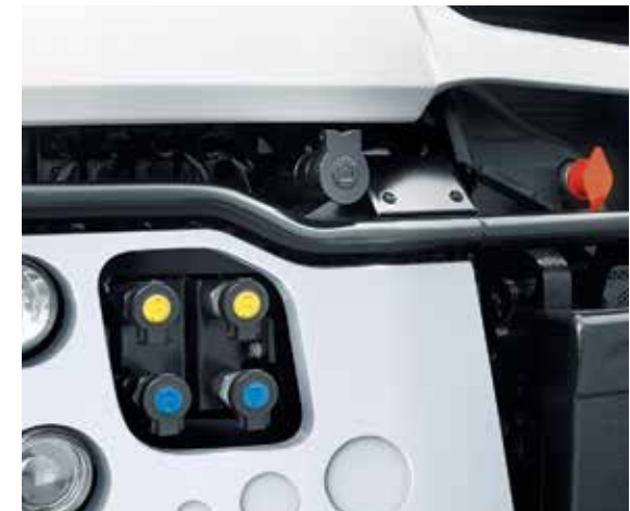
Hydraulic connections for up to four circuits are safely installed at the front and rear of the vehicle.
